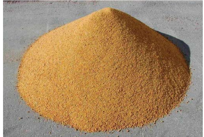
The enzymatic dry grind process developed by researchers at the University of Illinois reduces the volume of DDGS (above) by 65% to 70% and improves its nutritional characteristics. Photo courtesy of Distillers Grains Technology Council.
